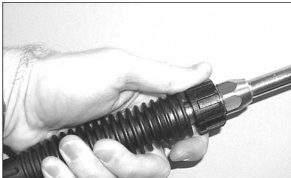
Figure 6 - Attach lance to gun
